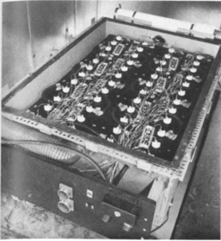
Fig. 2. 96 V test battery in the environmental chamber.
